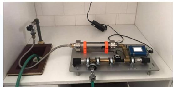
A device developed by researchers to measure the effect of IPS-treated water at different pressures on plant growth.
